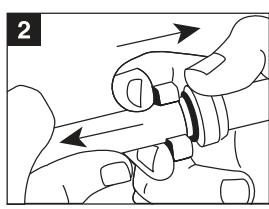
Place tool around pipe next to fitting. Press tool toward fitting while pulling pipe from fitting.
