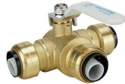
The Tectite by Mosack Group Push-To-Connect 3-Way Ball Valve is unique in that it can function as a diverter valve or mixing valve. It is the fastest, cleanest and simplest way to install or replace a 3-way ball valve on copper, CPVC, PE-RT and PEX piping systems without the use of tools, solder, open flame or glue. The quarter turn, single lever control allows for simple control of water flow in hydronic and potable water systems.
