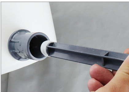
4. Push tool and ring into Snapport™ until it "SNAPS" in.
