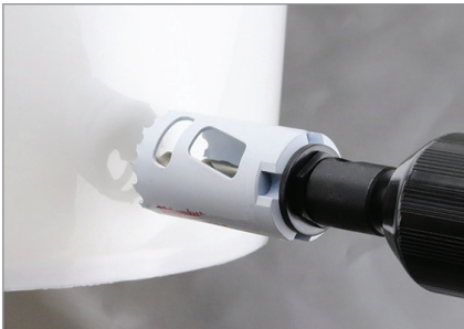
1. Drill a 1-1/8" hole into the vessel.
