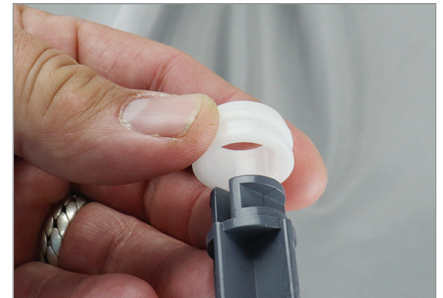
3. Place retainer ring on adjustment tool.
