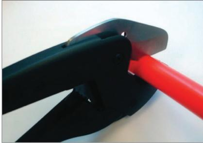
1. Cut tubing end squarely. Check for and remove any burrs.
