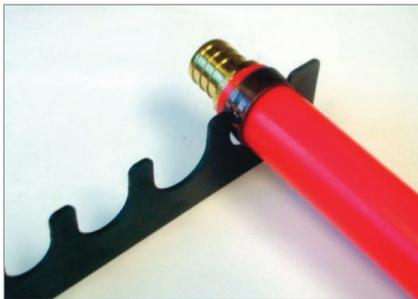
4. Check for proper crimp with the Go/ No-Go gauge.
