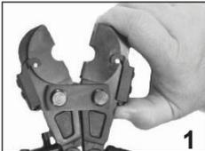
1. With the handles fully open, press side release spring upward until the hook is above the jaw pin.
