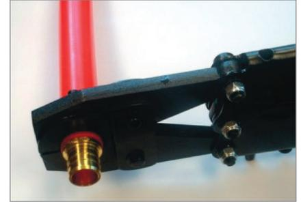
3. Place the crimping end of tool around the crimp ring and press the handles together.
