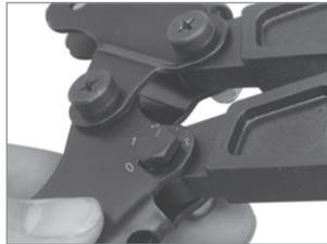
2. Push and rotate the screw. Increase the number for more crimp force. Decrease the number for less crimp force.
