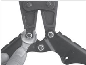
1. Open the handle, then loosen the nut on the screw with the numbers surrounding it.
