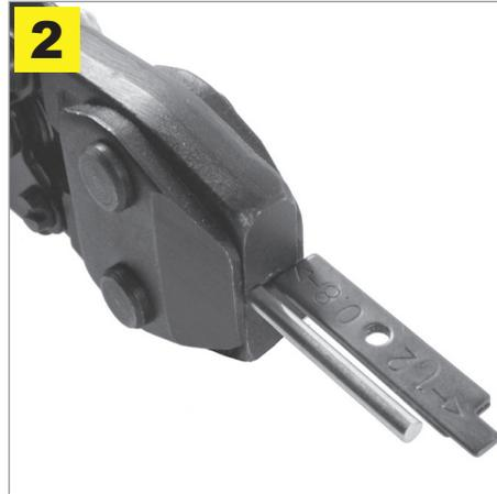
2. Use the Calibration Tool to gauge the jaw gap. Ideally, the jaw gap should be between 0.8 mm and 1.2 mm.
