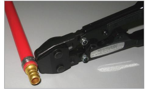
3. Place PEX pinch clamp nub between tool jaws and ratchet the clamp until the PEX Pinch Clamp Tool auto-releases. This action will assure that the PEX pinch clamp is fully engaged.
